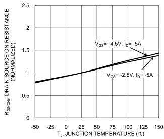
Figure 6. On-Resistance Variation with Junction Temperature
