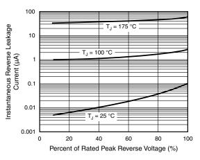
Fig. 5 - Typical Reverse Leakage Characteristics
