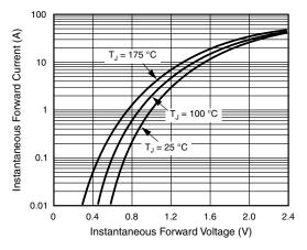
Fig. 4 - Typical Instantaneous Forward Characteristics
