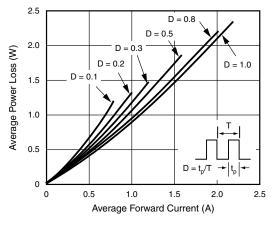
Fig. 2 - Forward Power Loss Characteristics
