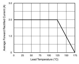
Fig. 1 - Forward Current Derating Curve
