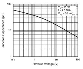
Fig. 6 - Typical Junction Capacitance
