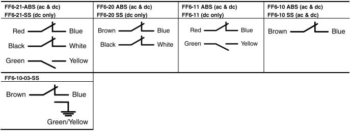
NOTE: Contact configurations show under closed condition for guard device.
