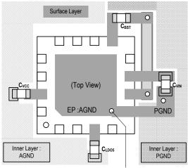
Connect the PGND to the AGND at single point directly under the IC
