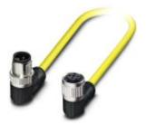
Sensor/Actuator cable, 4-position, TPE, yellow RAL 1021, Plug angled M12 SPEEDCON, A-coded, on Socket angled M12 SPEEDCON, A-coded, Cable length: 0.5 m
