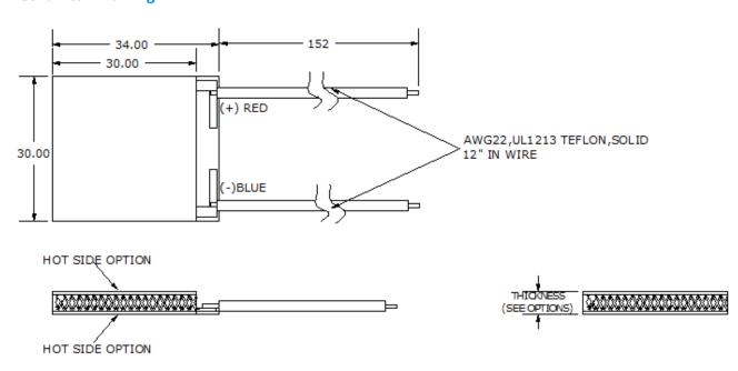
Ceramic Material: Alumina(Al2O3) Solder Construction: 232°C SbSn
