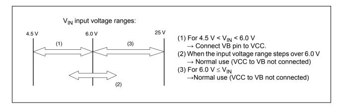
Note that if the I/O potential difference is not enough when used, use the actual machine to check carefully the operations at the normal operation, start operation, and stop operation. In particular, care is needed when the input voltage range over 6 V.
