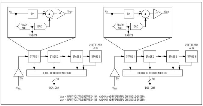
Figure 1. Pipelined Architecture—Stage Blocks
