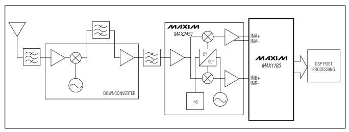
Figure 8. Typical QAM Application, Using the MAX1180
