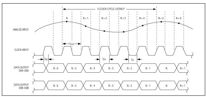
Figure 3. System Timing Diagram
