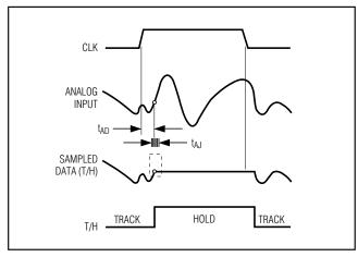
Figure 9. T/H Aperture Timing
