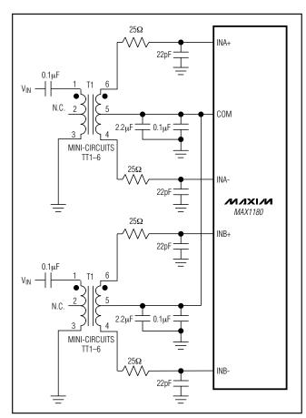
Figure 6. Transformer-Coupled Input Drive
