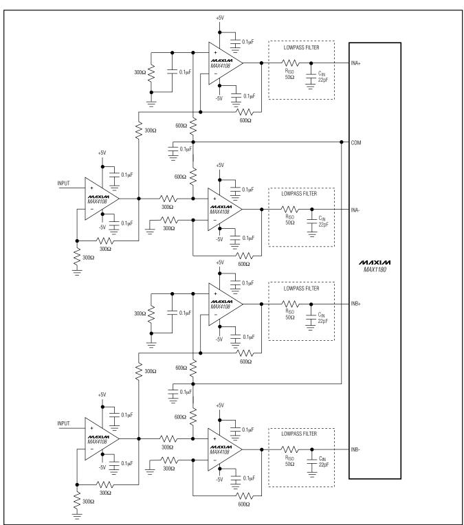
Figure 5. Typical Application for Single-Ended-to-Differential Conversion
