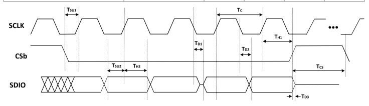
Figure 5.3. 3-Wire SPI Serial Interface Timing
