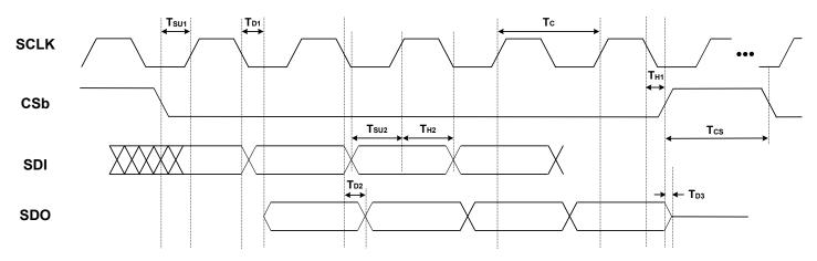
Figure 5.2. 4-Wire SPI Serial Interface Timing
