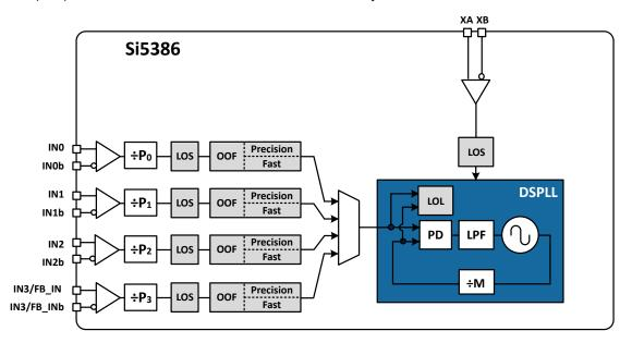
Figure 3.5. Si5386 Fault Monitors (Grade A)
