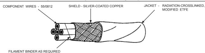
CABLE CONSTRUCTION DETAILS JACKET THICKNESS **OUTSIDE DIAMETER** CONDUCTOR SHIELD MAXIMUM PART NUMBER (in.) (in.) WEIGHT SIZE SIZE 1/ (lbs/1000 ft.) (AWG) (AWG) MINIMUM **NOMINAL NOMINAL MAXIMUM** 55/1852-28-\* 28 38 .006 .008 .128 .145 13.8 55/1852-26-\* 26 38 .006 .008 .141 .161 17.3 55/1852-24-\* 24 38 .006 .008 .155 .176 21.4 55/1852-22-\* 22 38 .006 .008 .192 .168 26.9 55/1852-20-\* 20 38 .006 .008 .190 .217 36.1
