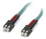
Assembled FO cable, zip cord cable, multi-mode fiberglass 50/125  $\mu$ m, OM3, plug: SC-RJ/SC-RJ, degree of protection: IP20, for installation in cable ducts or control cabinets, length: 2 m
