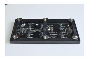
Lay them all out on a flat surface making sure their orientation is correct. Up arrow points up (duh) and each panel's output points towards the next's input.
