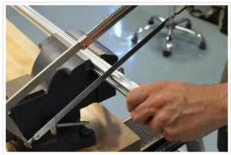
Mark the aluminum extrusions at 20.75" lengths and cut with a fine toothed hacksaw
