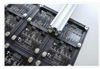
At this point the panels will have plenty of horizontal support, but need to be braced vertically. Now orient the outer oval T-nuts vertically and slide the 2 uncut single extrusions so that they line up with the top-most horizontal extrusion. They'll stick out a bit at the bottom.
