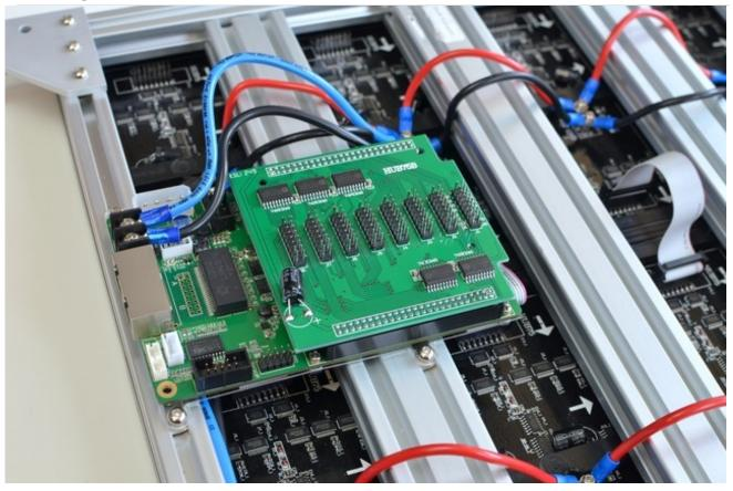
Once the receiving card has been mounted, plug the IDC breakout board in to the receiver card. Make sure that it's plugged in oriented as shown above.
