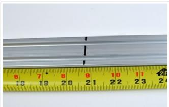
The frame is made up of five 20mmx40mm double slotted aluminum extrusions and four 20mmx20mm single slotted aluminum extrusions.
