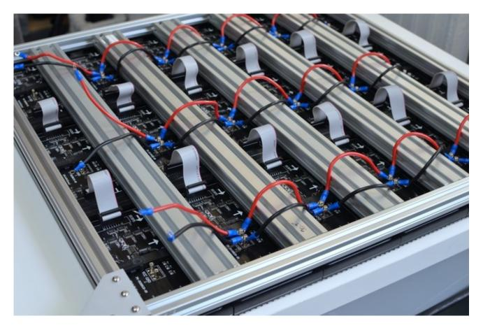
To provide power to the LED wall, I used a ATX computer power supply. Any 5V power supply that can provide more than 20 amps works too. ATX supplies work great because they're generally cheaper, and have standard & secure connectors.
