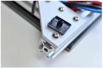
Place an end cap on the top and bottom of both single slotted extrusions to prevent it from sliding around.
