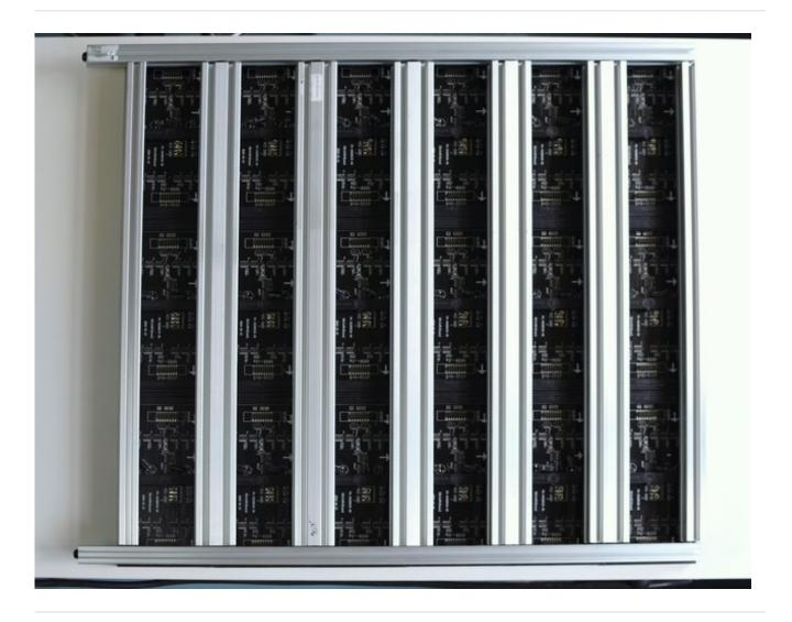
To secure the frame together, use 4 double corner braces, one in each corner. Drop 2 slim T-nuts into the extrusion's slot, lining them up with the corner braces holes. If the nuts need to repositioned
