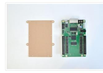
In order to mount the receiver card, a laser cut plate is needed to align the mounting holes with the extrusions and to keep it from shorting against the aluminum.
