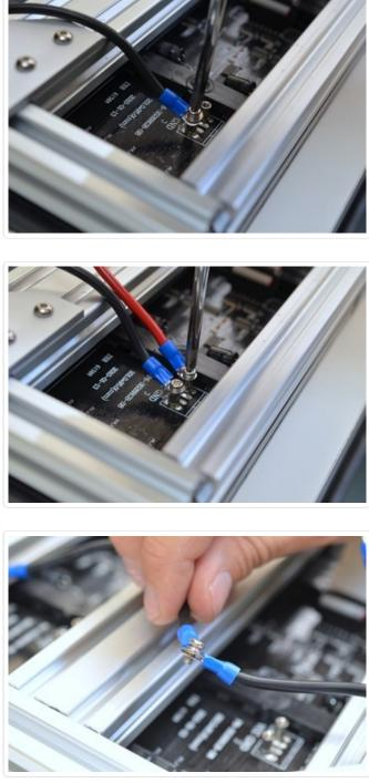
not as elegant to wire up the power. You can strip and solder the wires together instead.
