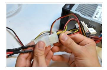
Before turning the power supply on, make sure all power is wired correctly. Seriously! This is 30A of 5V power, so you really really want to make sure its wired correctly.
