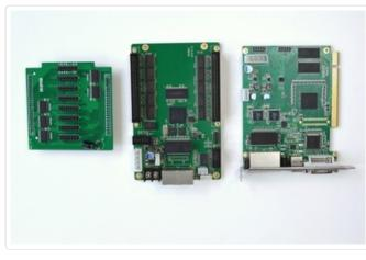
From left to right: IDC adapter for the receiver, receiver card, & sender card.
