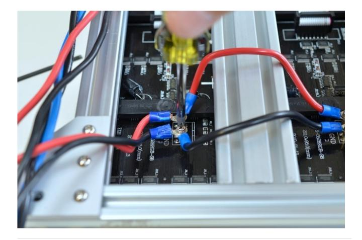
Run the power cables along the bottom aluminum extrusion and off to one side, zip tying them together to keep them tidy. Cut off the excess with diagonal cutters.
