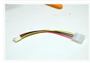
Cut a 4 Pin ATX power cable, keeping the larger connector, and strip the red and both black wires. Twist the two black wires together for redundancy.
