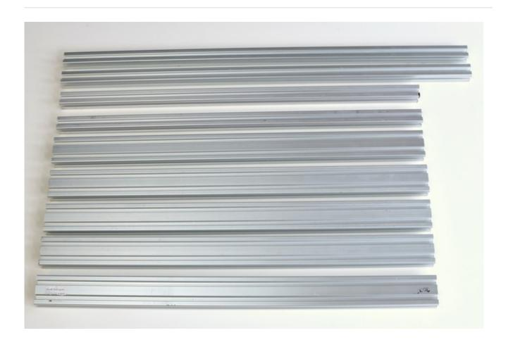
Orient the oval T-nuts horizontally and carefully slide them into the 20.75" double slotted extrusions, connecting the panels on top of one another. It should be tight, but if it won't slide any further, loosen up the screw a bit. Repeat this 4 more times. At the very top and bottom of the full wall, slide the 20.75" cut single extrusions to keep them even.
