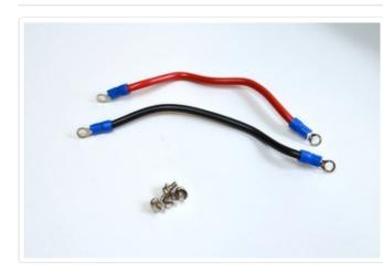
Each 16x32 panel comes with 2 cables and screws to provide power between them. To prevent voltage drops over long runs, each column will get its own 5V run of power.
