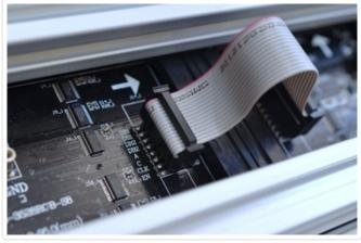
Connect each panel side by side with 12 short 16pin IDC's, leaving out the first input of each row (it will eventually be connected to the receiver board). Plug them in lining up the red wire of the IDC with the DR1 pin/up arrow on the board.
