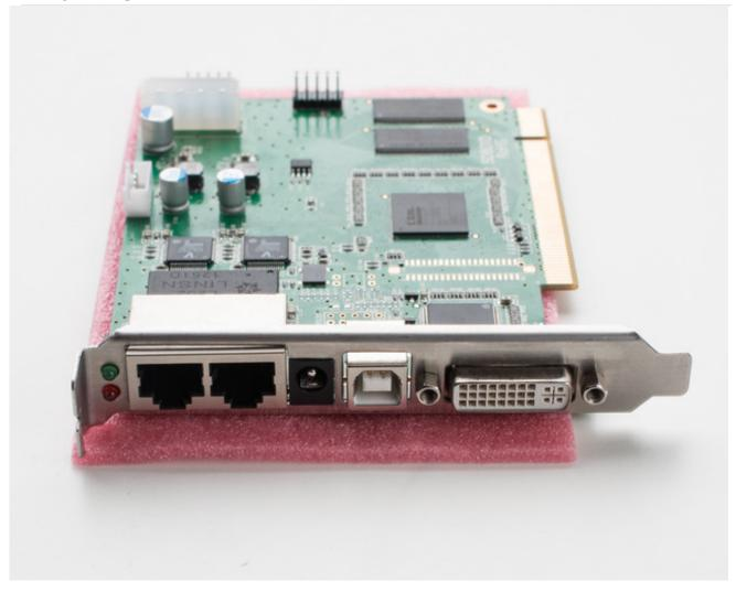
The sender card takes video input and spits it out via ethernet to the receiver card. Sending data over ethernet allows the video source to run long distances to the LED wall.
