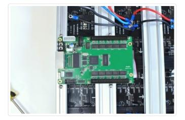
Jumper the 5V power from a nearby panel and screw it into the receiving card's power terminals. Depending on the positioning of the receiver card, you may need to make your own slightly longer power cables so that it'll reach.
